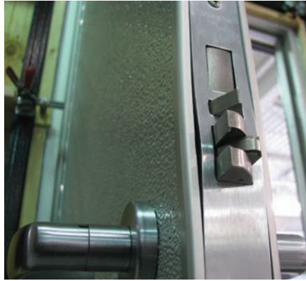
This door was tested to the ASTM F 1642 protocol for blast resistance protection. When subjected to force in the 5.5 to 6.5 psi range, the door was slightly damaged, as seen in the bend of the aluminum at the fastener, but remained operational.
