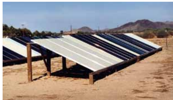
Special-Lite doors and door components weathering the intense heat and direct sunlight of the Arizona desert.
