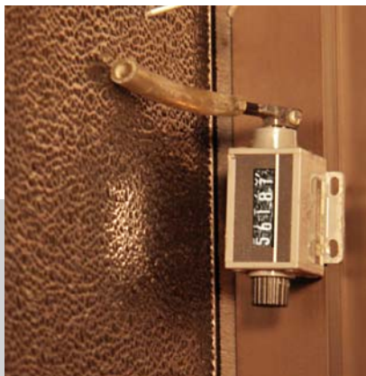
The cycles add up during the swing test of our SL-17 Door at Architectural Testing.
