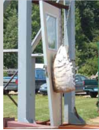
The sand bag impacts a door with bottom edge blocked.
